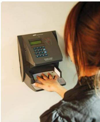
which captures a handprint. This is then fed directly to the software on the central server at the London HQ which compares the handprint against a stored profile to identify the employee and time stamps the record. This not only eliminates our crewhaving to complete time sheets, but the system is also foolproof, providing an accurate real time record of who is on site, when they arrived and when they completed their shift.
