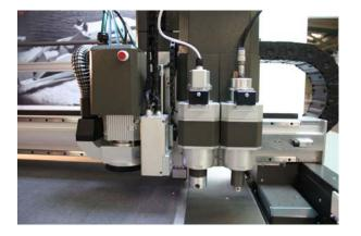
much larger patterns for all their sails and covers. The laser cuts with an accuracy of  $\pm 0.02$ mm, and as it's not in direct contact with the material, it means that even though it operates at speeds up to 1100mm/second, there's no dragging of the material so cutting is far more accurate than with a knife. Fully automated nesting algorithms allow patterns to be laid out to
